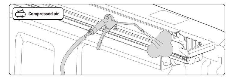
Remove dirt and debris using compressed air.
