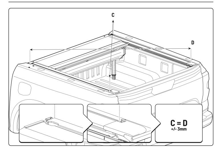
• Ensure the cross measurements are identical.
